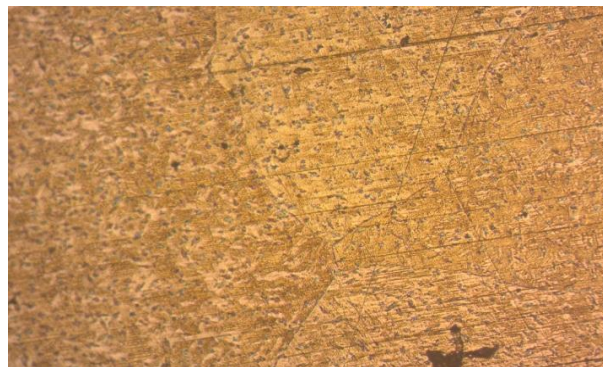
Figure 6: Inability of grain growth as a result of cooling from the mould.(x100)
