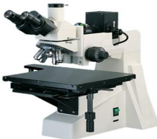
Figure 1: Optical Metallurgical Microscope used for the experiments (Federal University of Technology, Akure)
